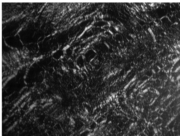
FIGURE 15 Planar cholesteric texture below Ch-I transition, 69°C.
