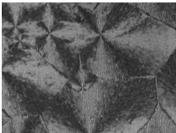
FIGURE 5 Well grown CC type domains in TGBA phase ( \times 100 ), 42°C.
